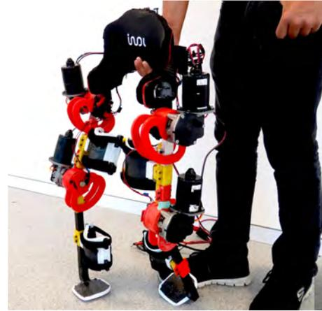
Fig. 1. ALICE Open Source Powered Exoskeleton without covers. This version shows joints constructed on red PLA, which were later substituted for black Onix (Nylon + Carbon Fiber). Four 12 [V], 26 [Nm] actuators are shown on four joints (two hip joints and two knee joints). Electronics are fit on the back (not seen) and the battery (not shown) is connected to the powered exoskeleton using a ~2 [m] cable, allowing for the device to weigh under 10 [kg].
