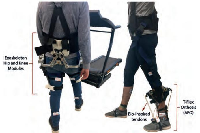
Fig. 1. AGoRA exoskeleton. On the left, the rigid parts of the exoskeleton are illustrated, as the hip and knee modules condition the motion of such joints to some degrees of freedom (DOF). On the right, the flexible component of this device (the ankle-foot orthosis T-Flex), used to enable all possible DOFs proper of the ankle joint.
