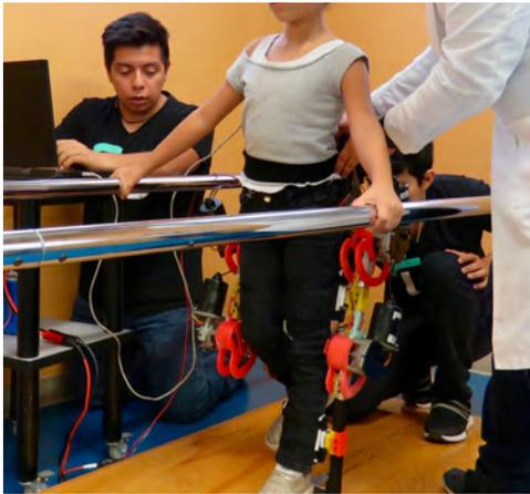
Fig. 2. Healthy Subject testing ALICE in its PLA version at Tecnológico de Monterrey's Hospital Zambrano Hellion. Tests typically require only one engineer (exoskeleton operator, left) and one medical doctor (right); however, initial tests with new subjects are normally performed by three research staff, to ensure subject safety and proper exoskeleton performance.
