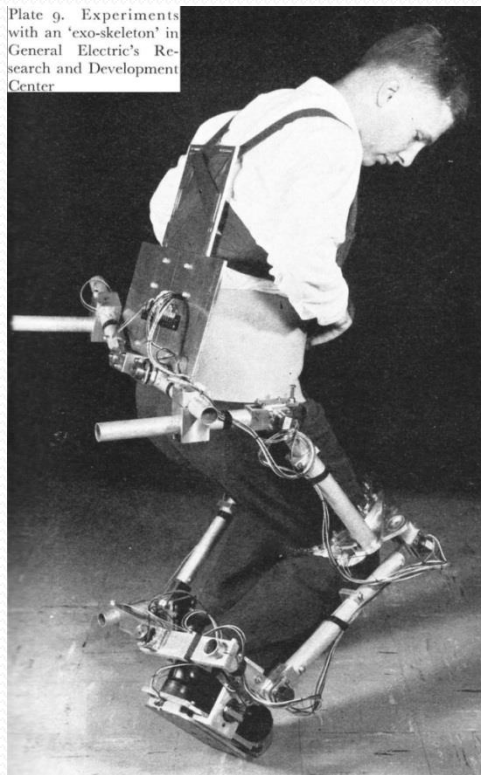
Hardiman I Exoskeleton (General Electric, 1965-71)
