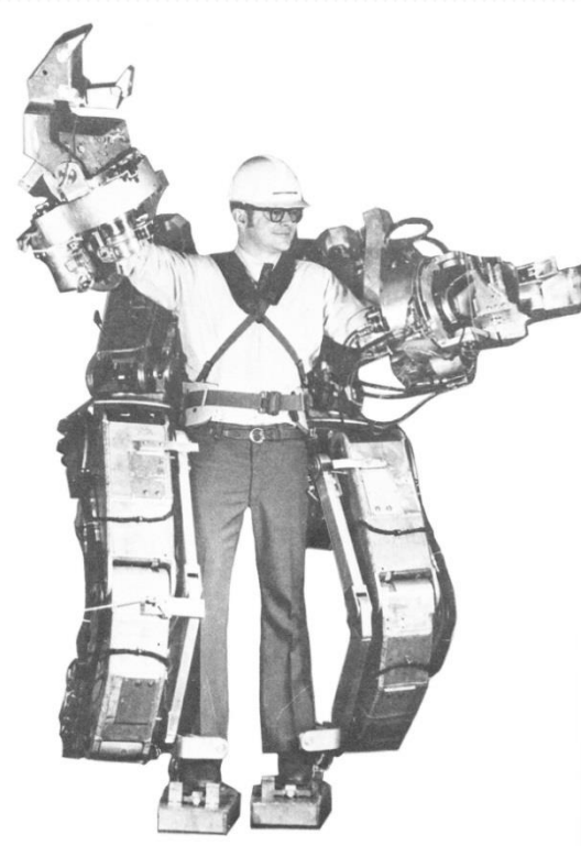
Hardiman I Exoskeleton (General Electric, 1965-71)
